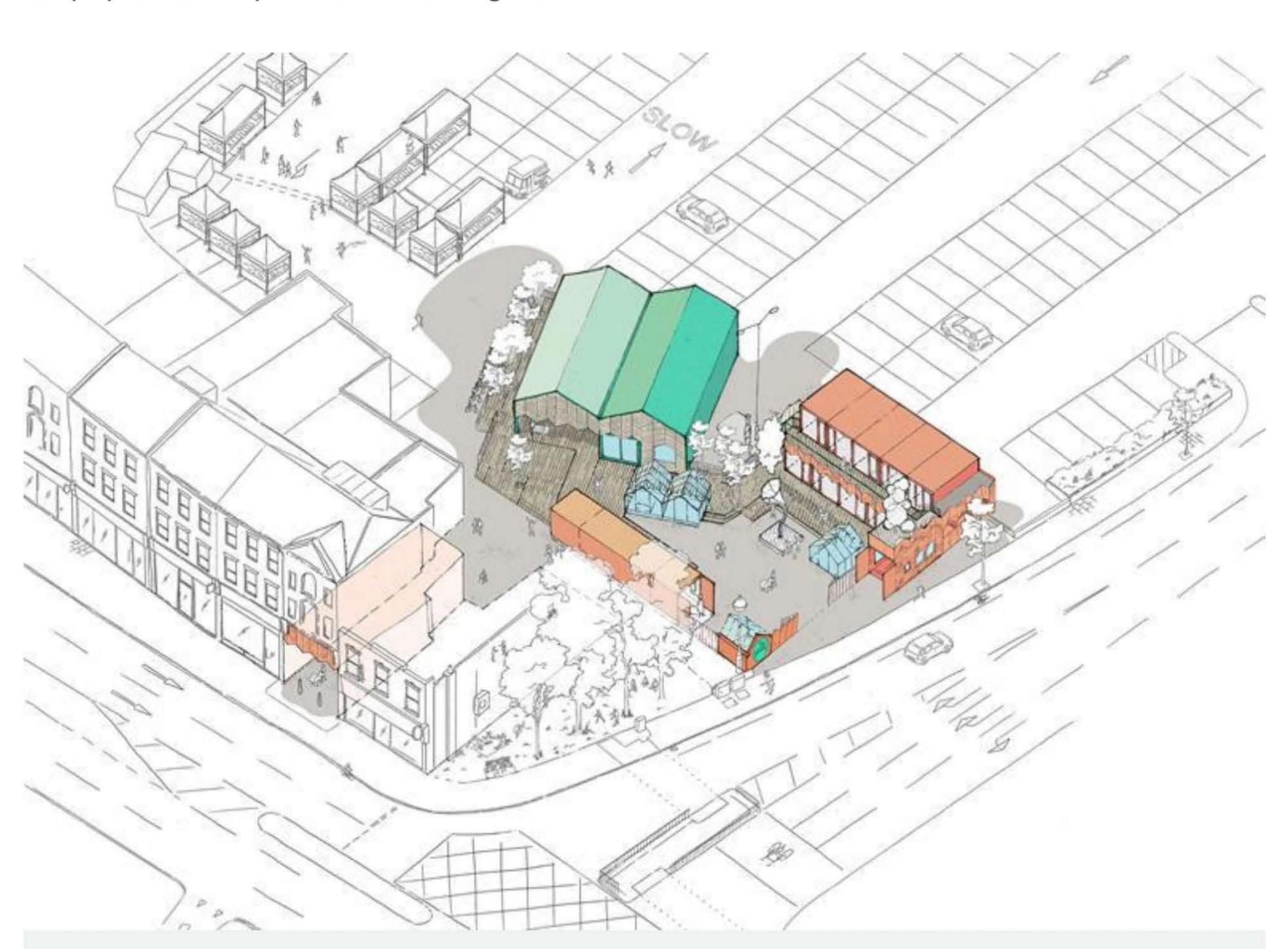
Sketch showing the three modular buildings arranged around the raised courtyard, with container galleries, glasshouses and planted screening on the site
